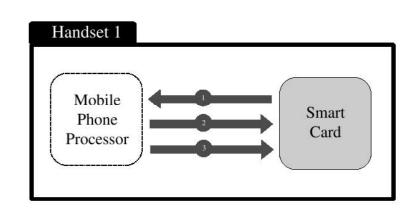
• The smart card is ready The phone sends a command APDU The card sends a response APDU
